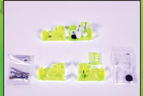
FIGURE 6. Build a left and right motor gearbox. The gearboxes are identical until the drive axles are installed.
